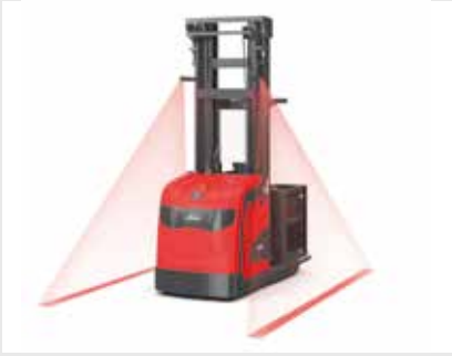
Red warning lines for safe operation
